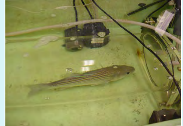
Striped bass placed into a respirometer for determining metabolic rate
