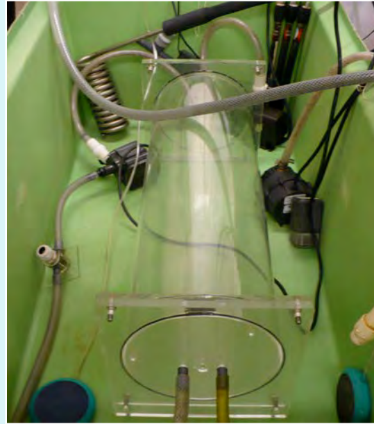
Respirometer (acrylic tube), pumps, chiller and heaters in an empty aquarium
