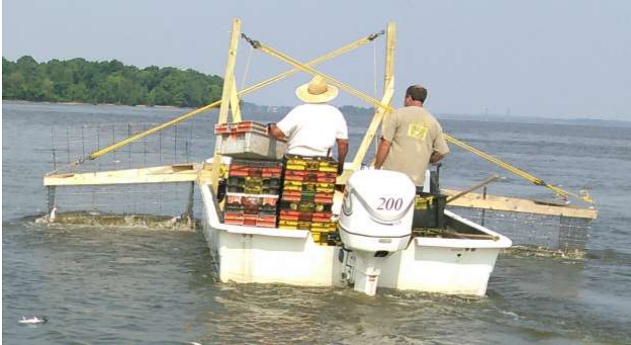
Figure 3. Picture of the butterfly skimmer setup on the 27' Carolina skiff. The boat is actively operating during low-frequency electrofishing operations.
