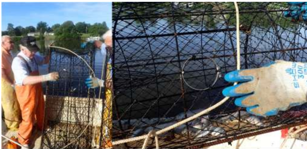
Figure 3. Adjustable stainless steel hose clamps sewn into the pot outer webbing served as cull rings which could be adjusted to various testing diameters.
