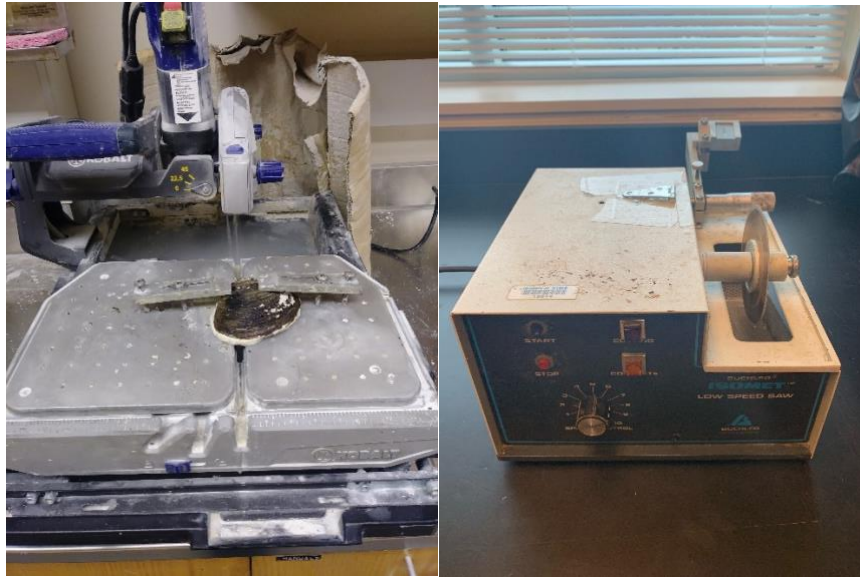
Figure 3: Examples of tile saw and slow speed saw used to cut shells.
