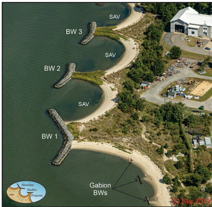
Figure 6-14. Aerial photo taken in September 2019 showing VIMS West nearly 9 years after construction.
